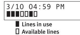
If your system has 16 or fewer lines, each block on the bottom line of the display will represent an individual line (as in the seven-line example, above). Incoming calls usually are assigned beginning with Line 1 at the far-left line indicator. Outgoing calls are assigned from the highest numbered line beginning at the far right.
